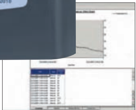
OM-SQ-SOFT, Windows software (included with OM-SQ2010 data loggers) displays data in graphical or tabular format.
