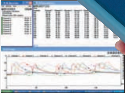
TC-08 Windows software displays data in graphical or tabular format
